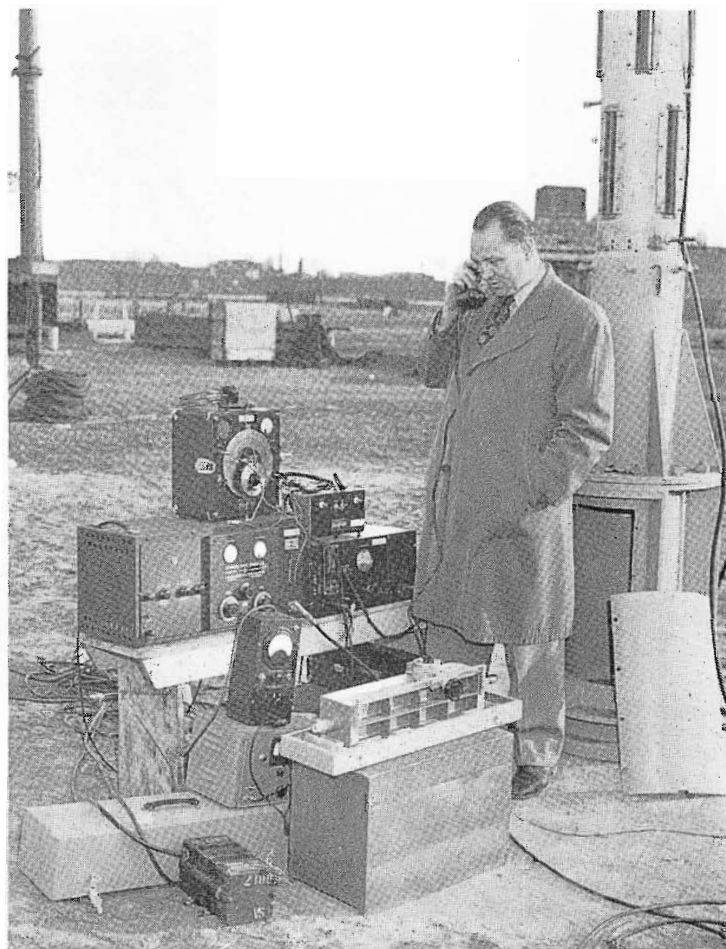
FIG. 8 (above, right). TEST SETUP at Camden is shown in this view. Antenna is mounted on rotatable base and fed power by signal generator at extreme left. Pickup antenna on roof of small building at right feeds recording equipment located in the building.
